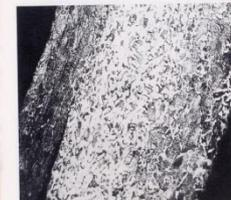
Figure 49. Sample from armor in Figure 48 (x 140). Cross-section. A band of pearlite, some of which has been distorted, next to a band of mixed ferrite and pearlite.
