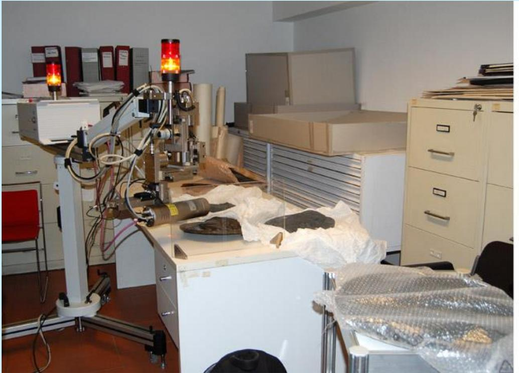
Rhodium tube with 1 mm collimator at 50 keV and 700  $\mu$ A
